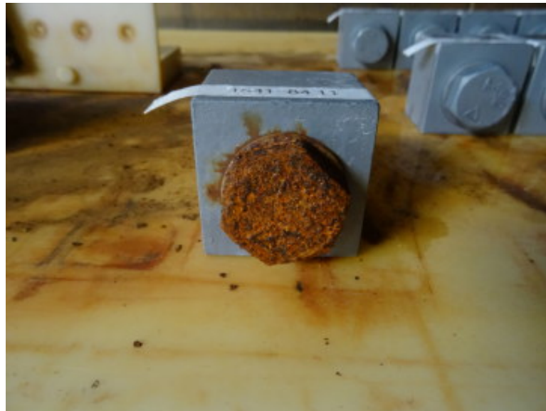
Figure 15 – Bare sample after 20 cycles
