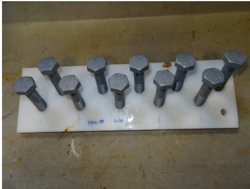
Figure 12a – 3/4 inch specimen bolts after 1000 h of salt spray exposure
