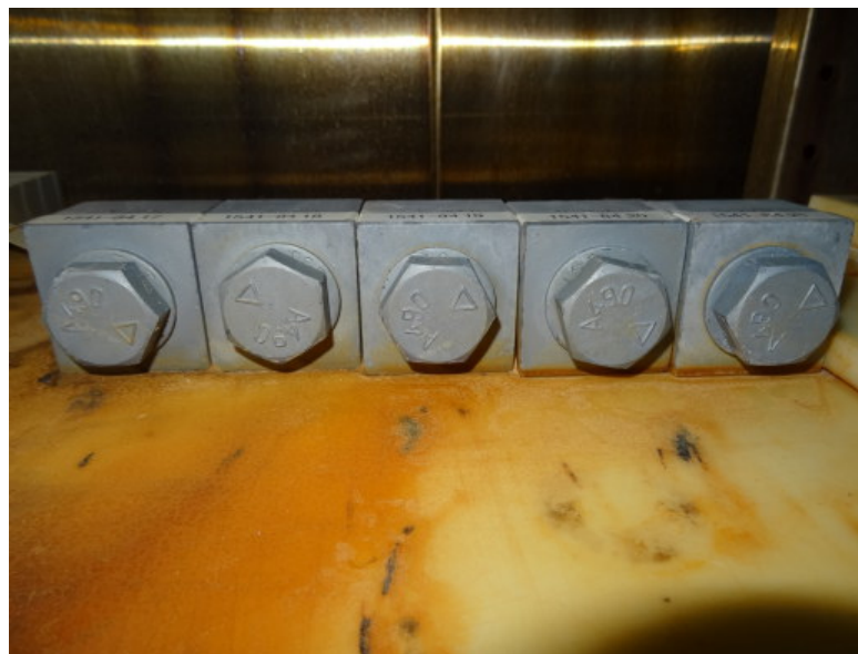
Figure 17 – Delta Protekt® KL 105 coated - Turn -of nut tightened - after 120 cycles
