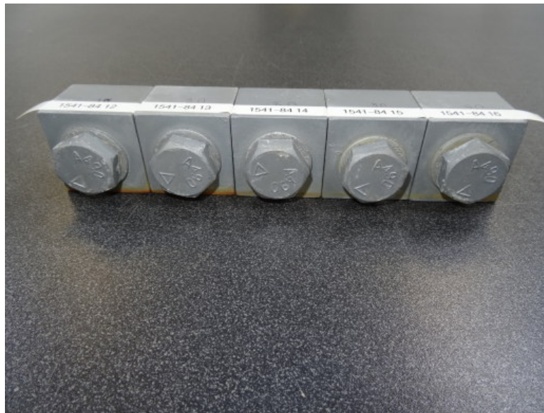
Figure 16 – Delta Protekt® KL 105 coated - Finger tightened - after 120 cycles
