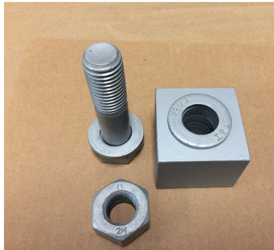
Figure 13 – test components used for cyclic testing, each assembly comprising one bolt, one nut, two (2) washers, all assembled in the test block
